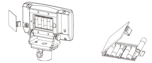
**NOTE!** Do **not** use rechargeable batteries. If you do, the batteries should be charged in an external charger. The scale adapter cannot charge the batteries when they are in the scale.
