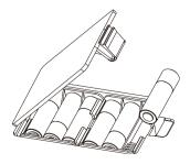
**NOTE!** Do **not** use rechargeable batteries. If you do, the batteries should be charged in an external charger. The scale adapter cannot charge the batteries when they are in the scale.
